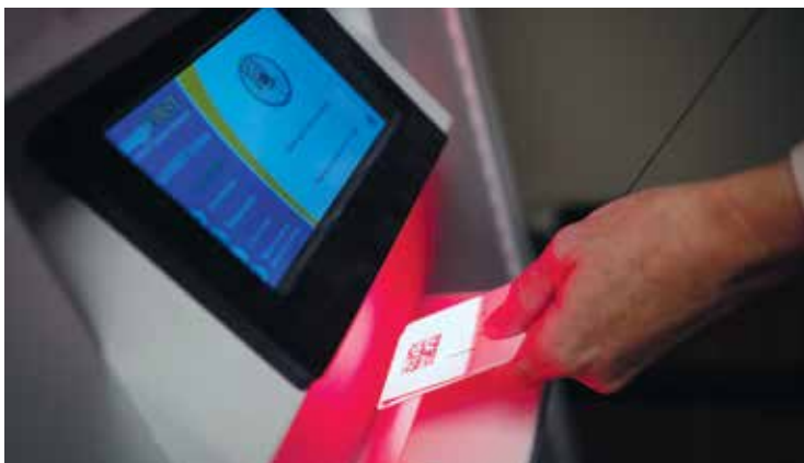
Staff members scan their badge, and the dispenser opens, noting the employee's specific size being removed.
